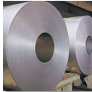
Coated sheets (used in cars, electrical appliances, cans, etc.)
